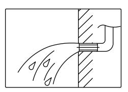
In order to avoid the obstruction of faucet, must to clean the impurigites and sludge of pipe, before assembly.
