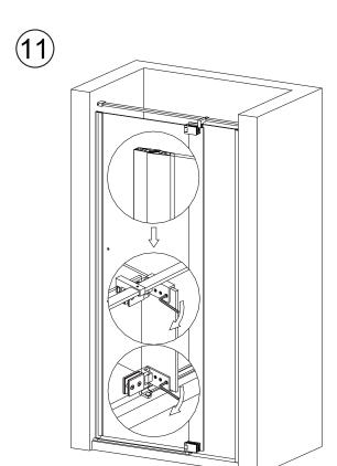
Adjust the moving glass, make sure the magnetic stripe adsorbed tightly.
