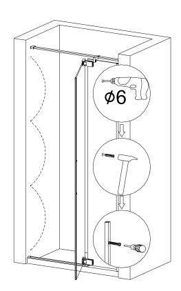
Drill a \$6\$ hole. Knock in the \$6\$ Rubber. Lock the 8×8mm square tube tightly by a ST4×30 tapping screw.
