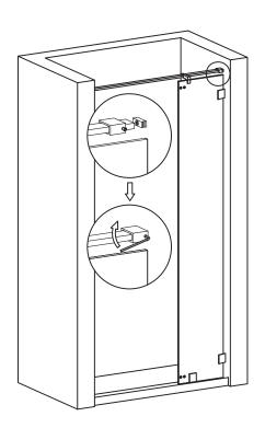
Install the draw bar parts. Tight the tube seat with a 3 mm hexagonal key.
