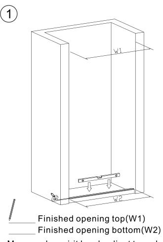
Measure by spirit level, adjust to make sure the installed position is horizontal.
