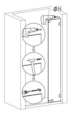
Drill a \$\phi 8\$ hole. Knock in the \$\phi 8\$ Rubber. Lock the tube fixing part tightly by a ST5×35 tapping screw.
