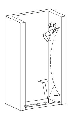
Drill a hole by an  $\phi$ 6 driller, Knock in the 6mm expansion screw.
