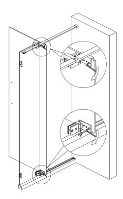
Tight the moving glass with a 4 mm hexagonal key.
