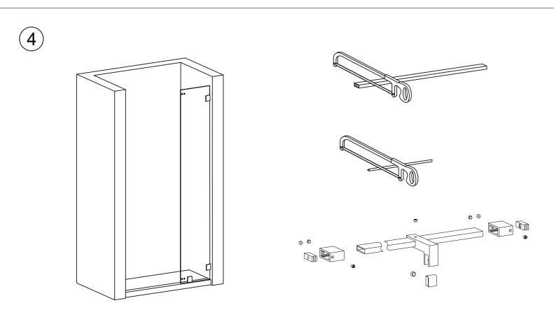
Saw cutting the suitable length of the stainless steel tube and Aluminum water bar on the basis of practical need. Assembly the draw bar parts.
