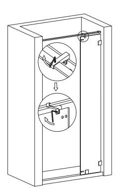
Tight the clamp with a 3 mm hexagonal key.
