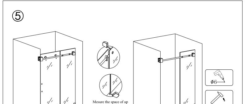
1. Put two plastic sliding cover and movable glass onto the base stone. Measure the space between the movable glass and fixing glass, make them vertically. Mark the sliding cover position by pencil, take off movable glass and sliding cover, then drill a hole by a Ø6 driller and insert with inflatable rubber.
