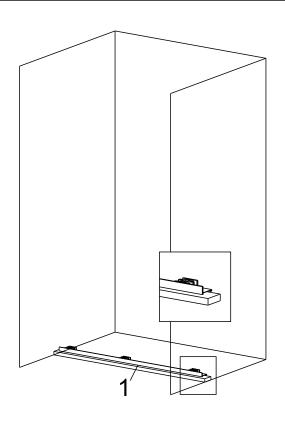
Put the down-rail to the installation position. Make sure that down-rail is in the center position, leave some space at both ends in order to install side column.
