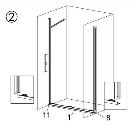
Insert the right and left column to the down-rail. Pay attention to the bottom slotting direction. Exchange the side column if the slotting direction is wrong.
