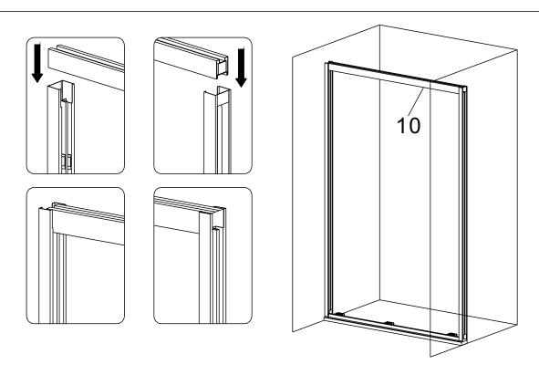
Make the both ends of the uppper rail into the slot of the side column, push down hard to make it flatten. After install the up-rail, adjust the length of both ends, so that the length of which rail of the column is the same.
