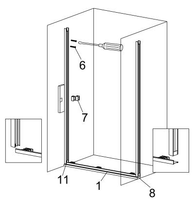
Put the down rail to the base stone, and put the left and right side columns to the down rail, measure it horizontally by spirit level.
