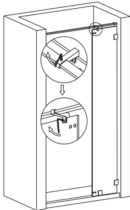
Tight the clamp with a 3 mm hexagonal key.
