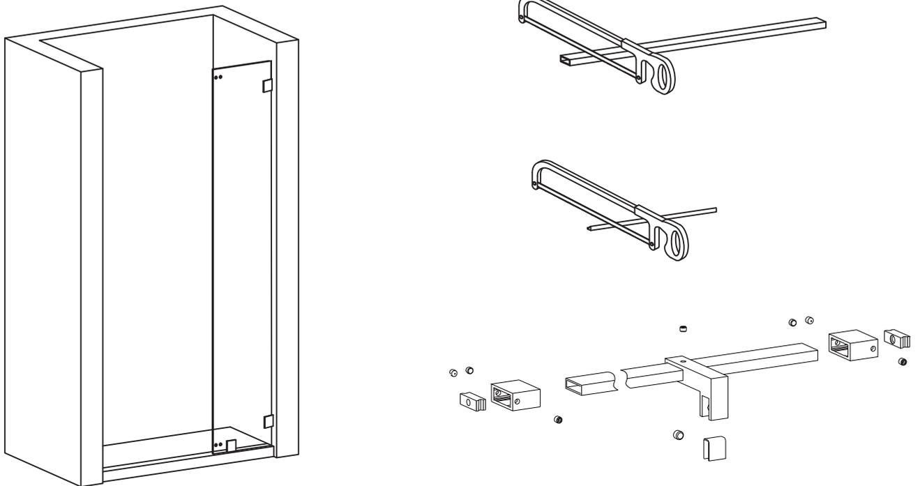
Saw cutting the suitable length of the stainless steel tube and Aluminum water bar on the basis of practical need. Assembly the draw bar parts.
