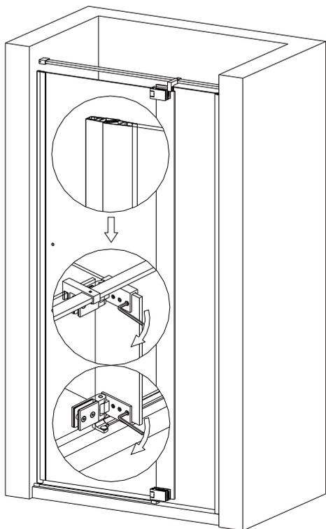
Adjust the moving glass, make sure the magnetic stripe adsorbed tightly.
